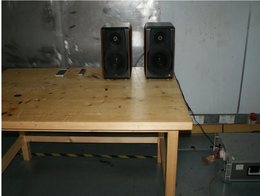
Photograph 1: Set-up for Conducted Emission on AC Mains
