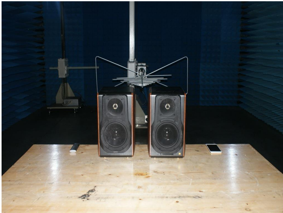
Photograph 2: Set-up for Radiated Emission, below 1GHz
