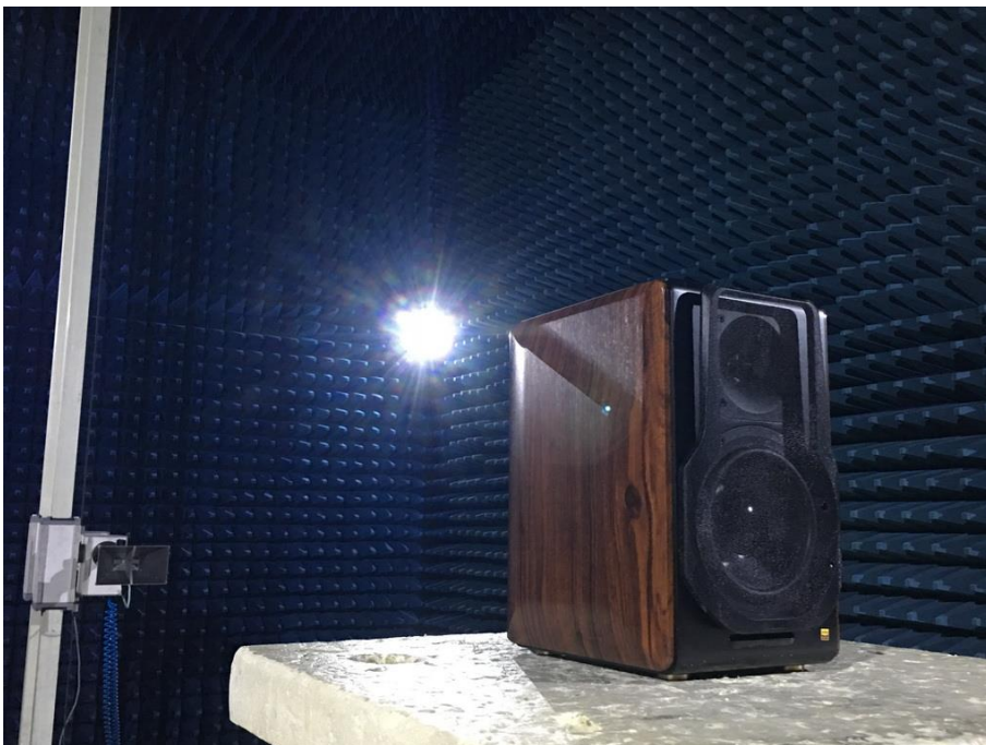
Photograph 6: Set-up for Radiated Spurious Emission, 1GHz - 18GHz
