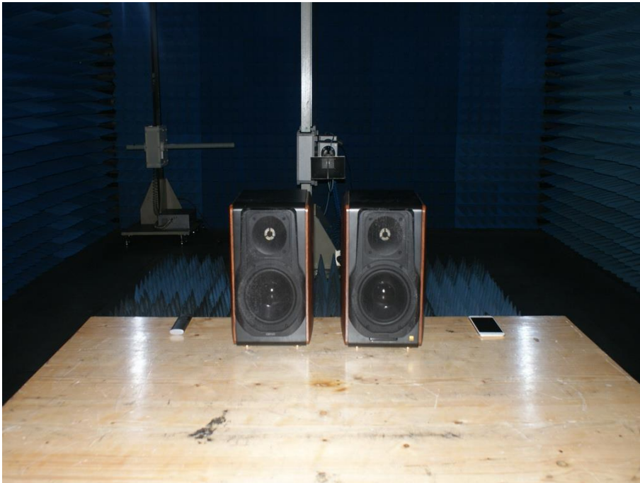
Photograph 4: Set-up for Radiated Spurious Emission, 9KHz - 30MHz
