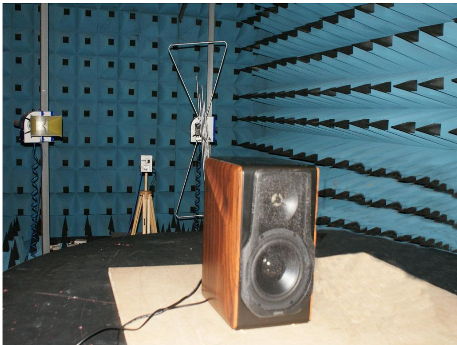
Photograph 8: Set-up for Radiated Spurious Emission, 26.5GHz - 40GHz
