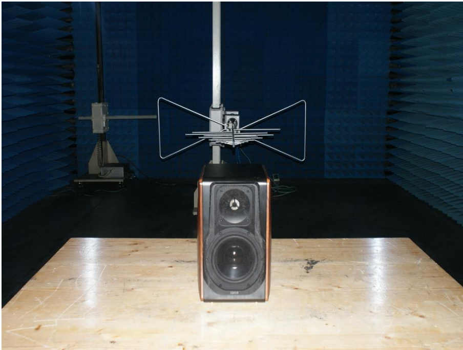
Photograph 5: Set-up for Radiated Spurious Emission, 30MHz - 1GHz
