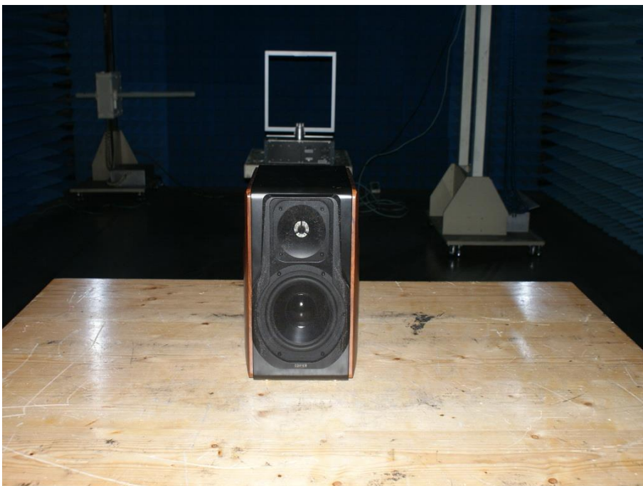
Photograph 4: Set-up for Radiated Spurious Emission, 9KHz - 30MHz
