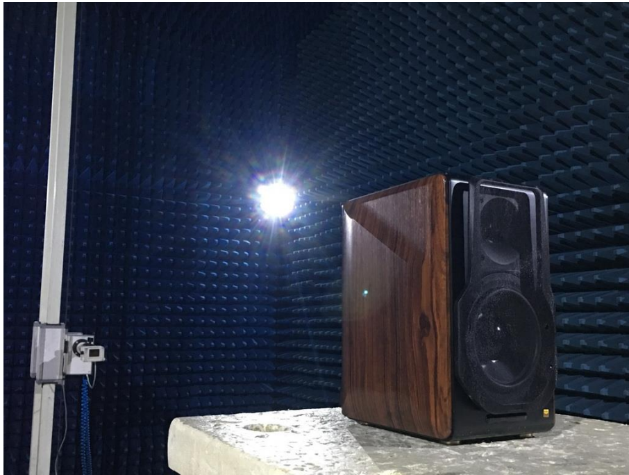
Photograph 7: Set-up for Radiated Spurious Emission, 18GHz - 26.5GHz
