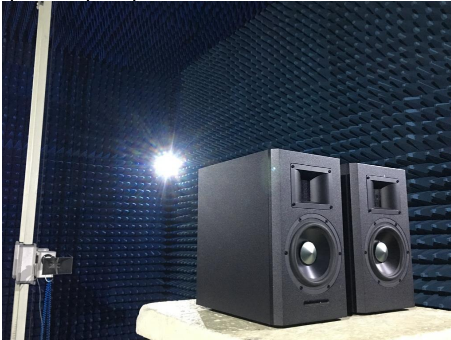
Photograph 4: Set-up for Spurious Emissions for 18 - 26.5GHz
