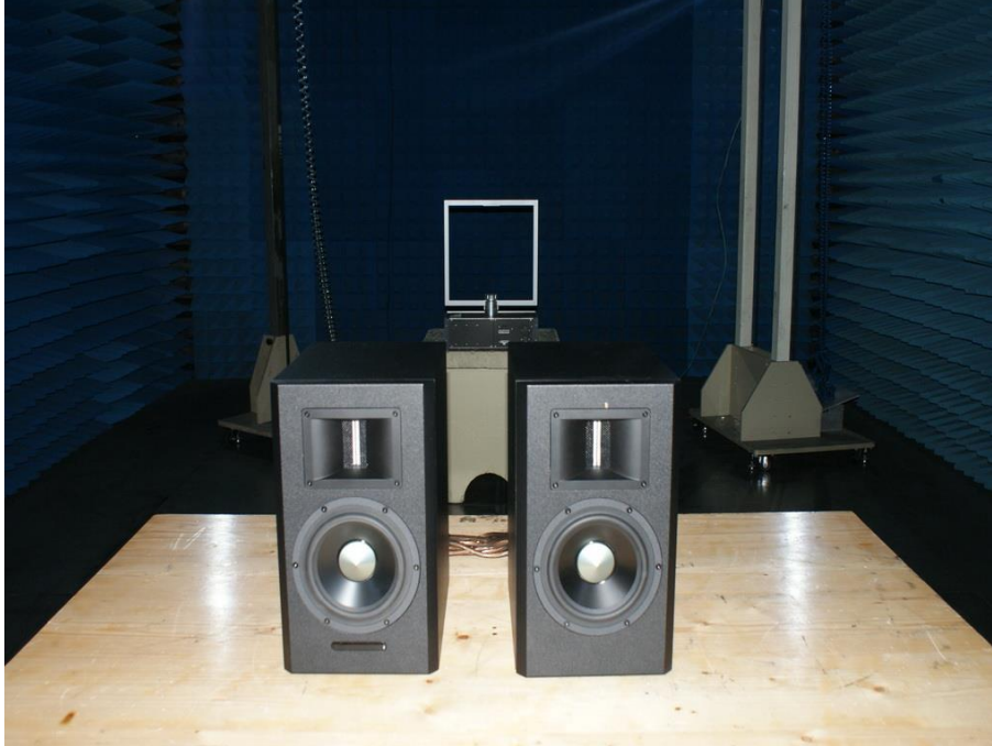
Photograph 2: Set-up for Spurious Emissions for 30 - 1000MHz
