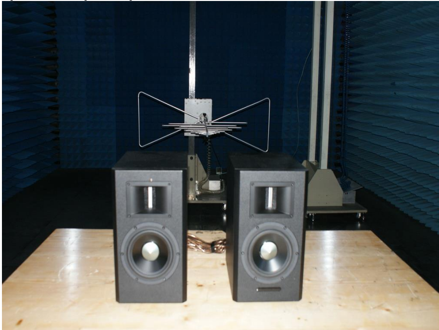
Photograph 2: Set-up for Spurious Emissions for 30 - 1000MHz
