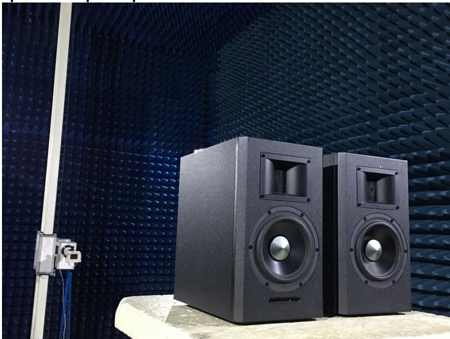
Photograph 4: Set-up for Spurious Emissions for 18 - 26.5GHz
