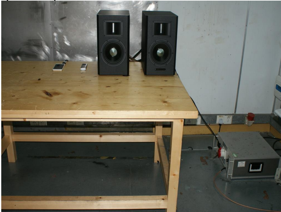
Photograph 5: Set-up for Conducted Emissions
