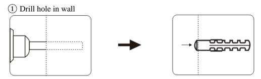
Drill 4 holes (Depth: 40mm/1.5", Hole size: 8mm/1/4") in the wall using the wall mount bracket as a template, then knock wall anchor into holes.
