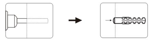
For each rear surround speaker, drill 2 holes (Depth: 40mm/1.5", Hole size: 8mm/1/4") in the wall using the bracket as a template, then knock wall anchor into holes.
