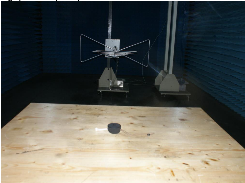
Photograph 2: Set-up for Spurious Emissions for 30 - 100MHz
