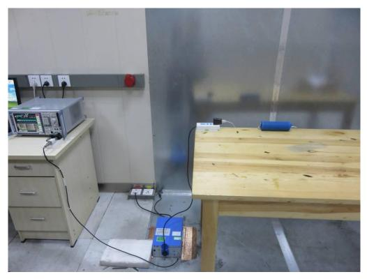
FCC RADIATED EMISSION TEST SETUP
