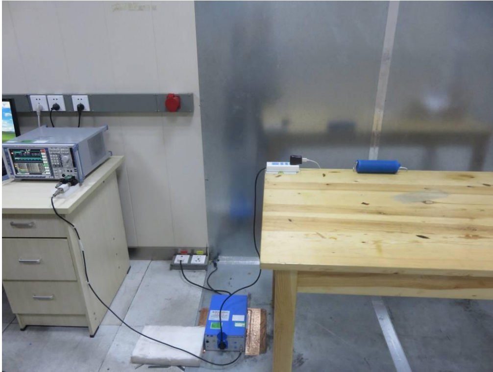
FCC RADIATED EMISSION TEST SETUP
