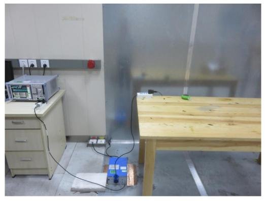
FCC RADIATED EMISSION TEST SETUP
