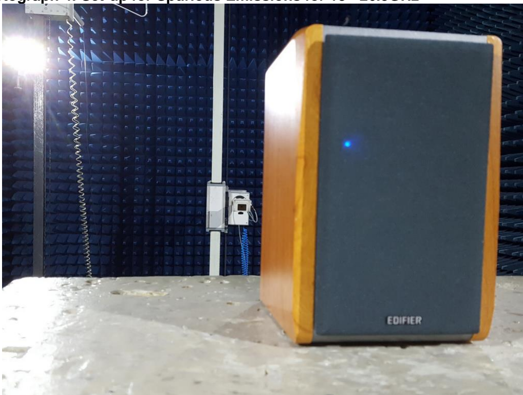
Photograph 4: Set-up for Spurious Emissions for 18 - 26.5GHz
