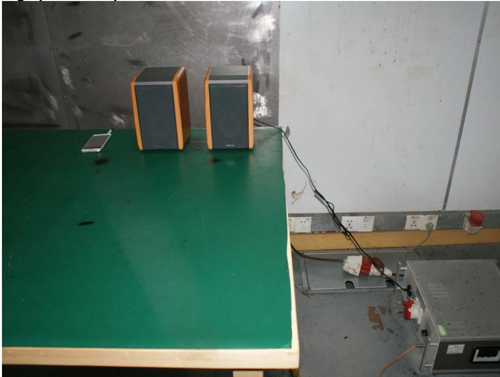
Photograph 6: Set-up for Radiated Emissions
