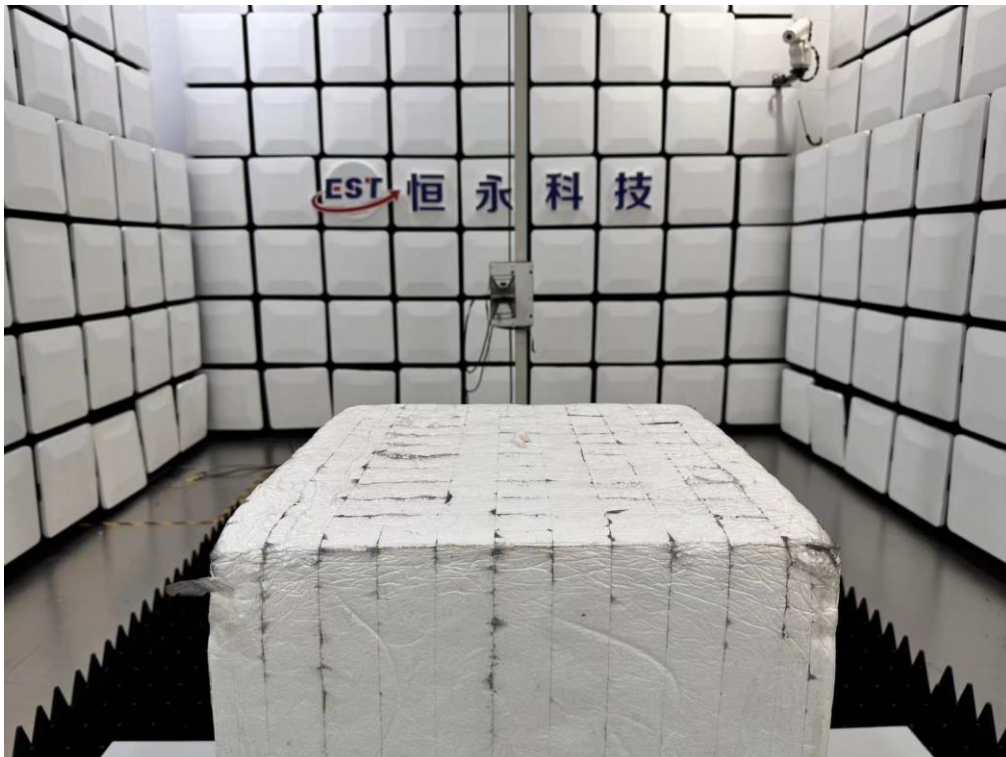
Radiated emission test: Above 1GHz
