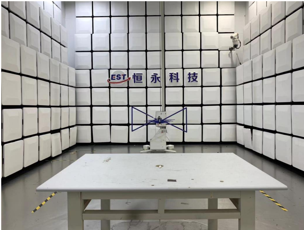
Radiated emission test: Below 1GHz
