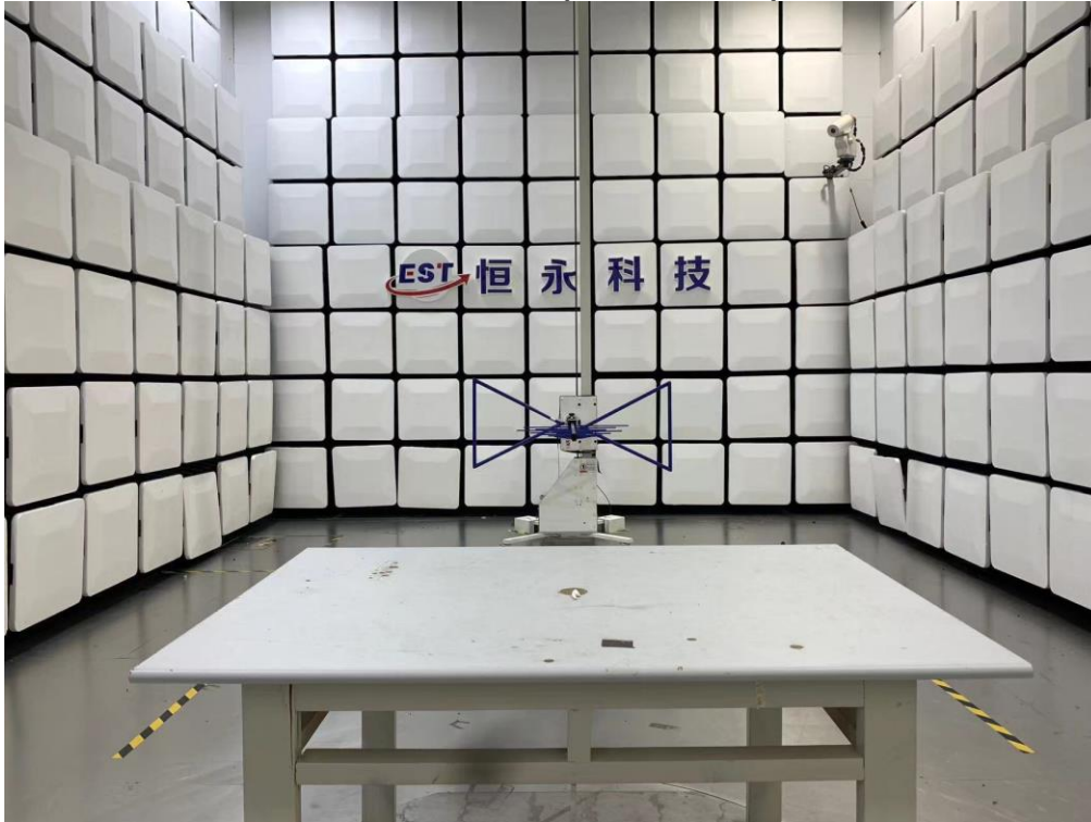
Radiated Test (Below 1GHz)
