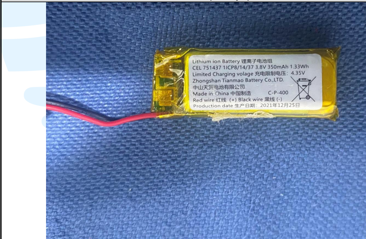
EUT Photo (Battery 2)
