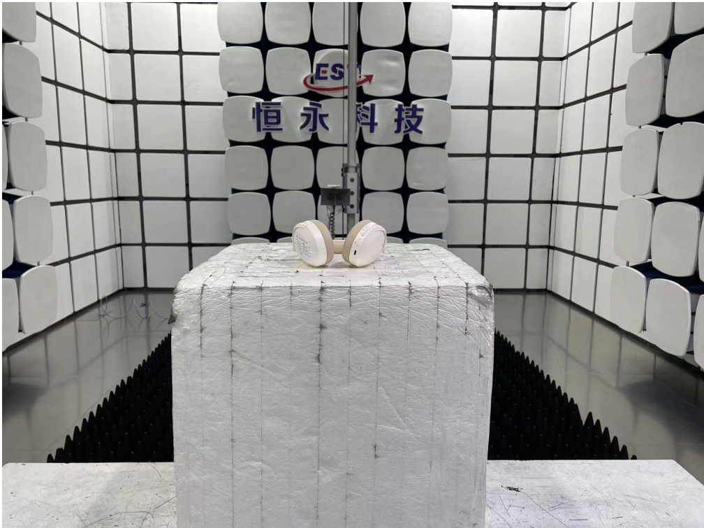
Radiated emission test: Above 1GHz
