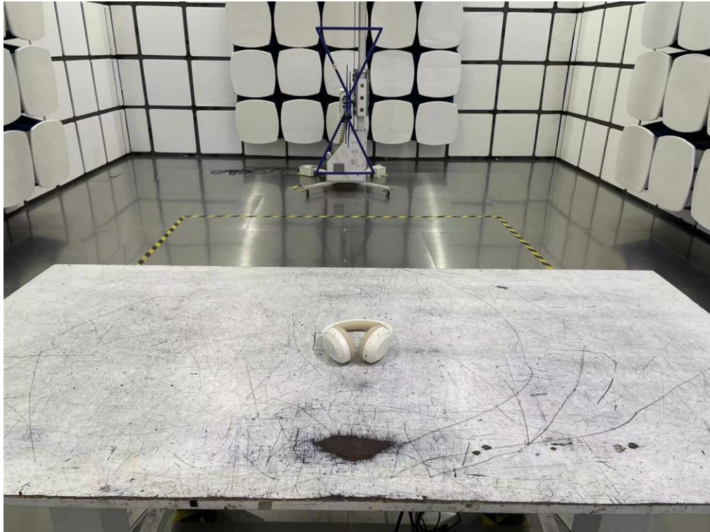
Radiated Test (Below 1GHz)
