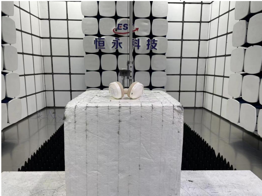
Radiated Test (Above 1GHz)
