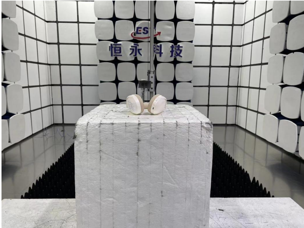
Radiated Test (Above 1GHz)
