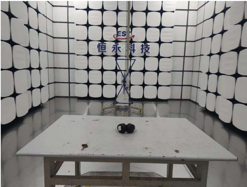
Radiated emission test: Below 1GHz
