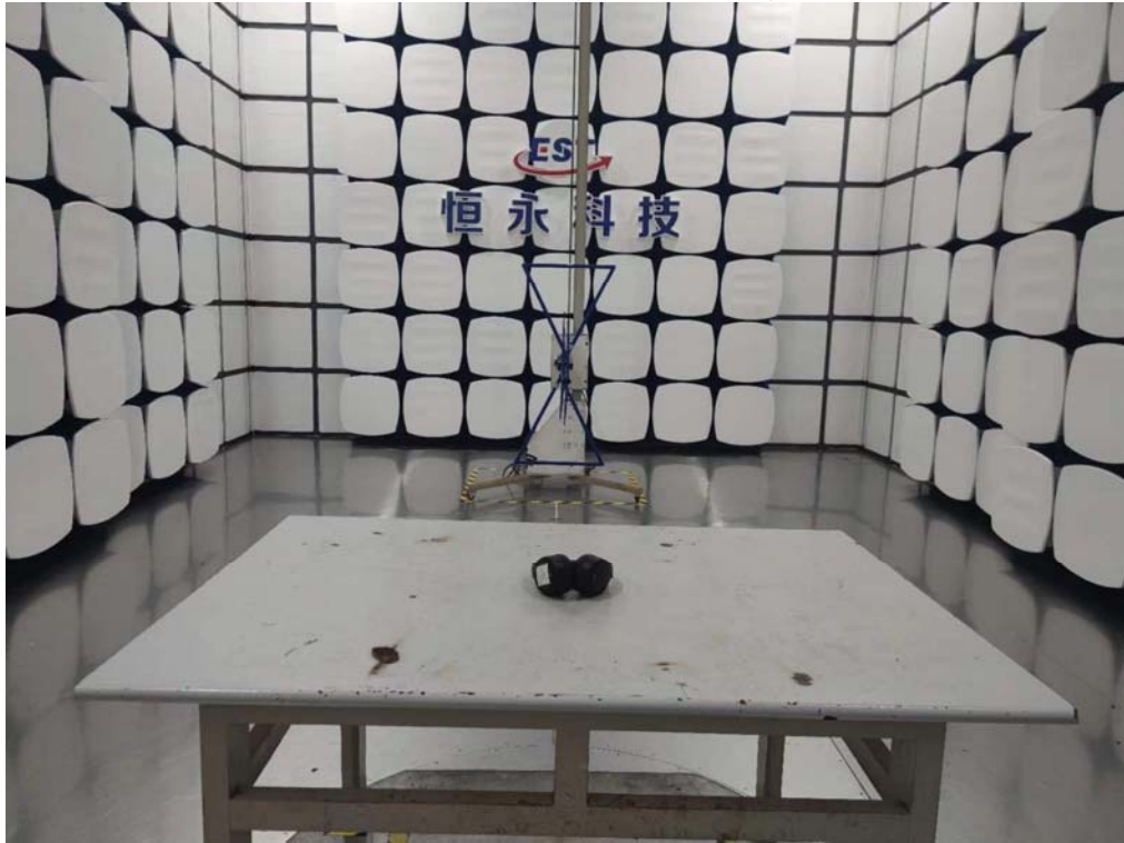
Radiated Test (Below 1GHz)
