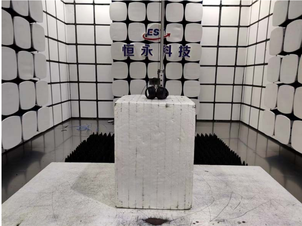
Radiated Test (Above 1GHz)
