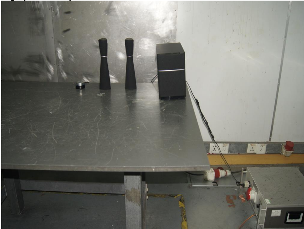
Photograph 2: Set-up for Spurious Emissions for below 30MHz
