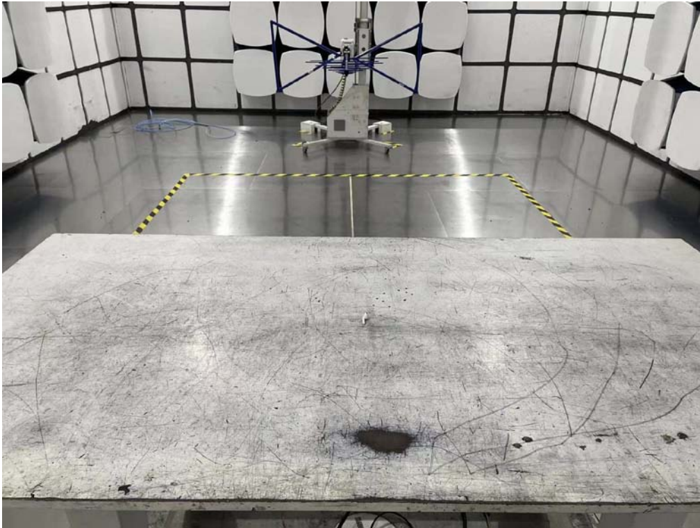
Radiated Emission Test: Below 1GHz
