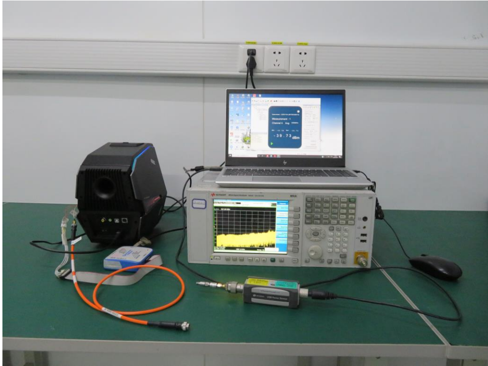
Description: Radiated Spurious Emission Test Setup for below 1GHz
