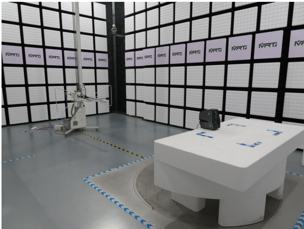
Description: Radiated Spurious Emission Test Setup for below 1GHz
