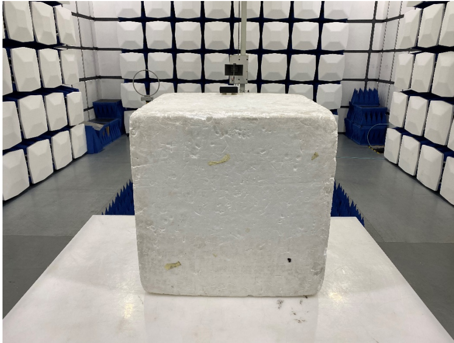
Photograph 3: Set-up for Radiated Spurious Emission, above 1GHz
