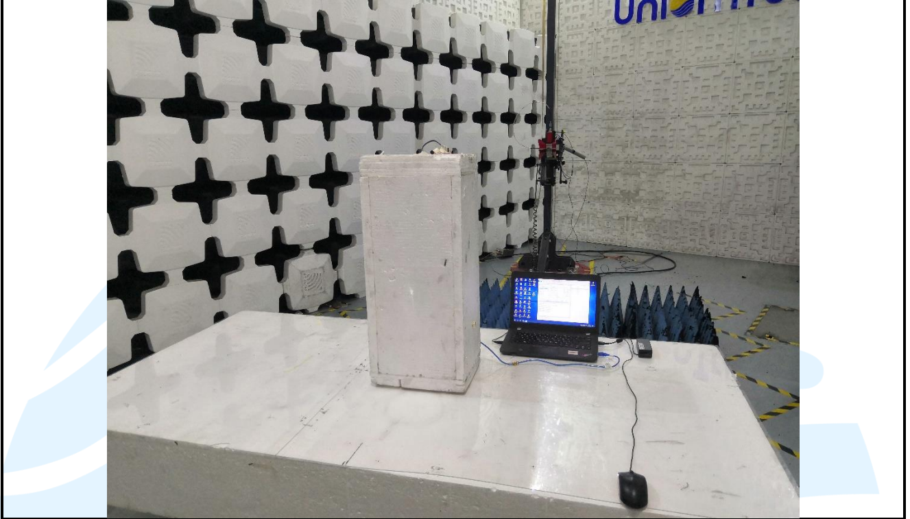
Radiated emission Test Setup (Above 1 GHz) -Left
