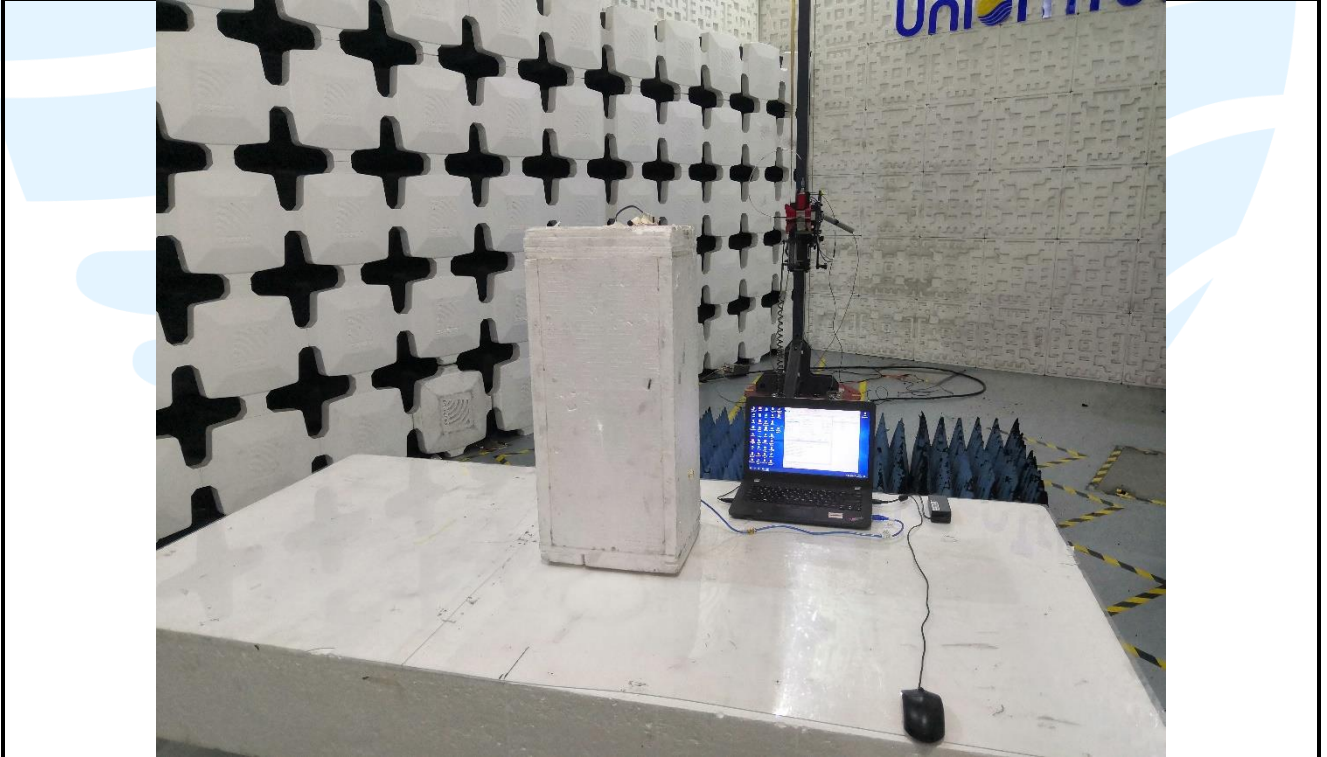
Radiated emission Test Setup (Above 1 GHz) -Right
