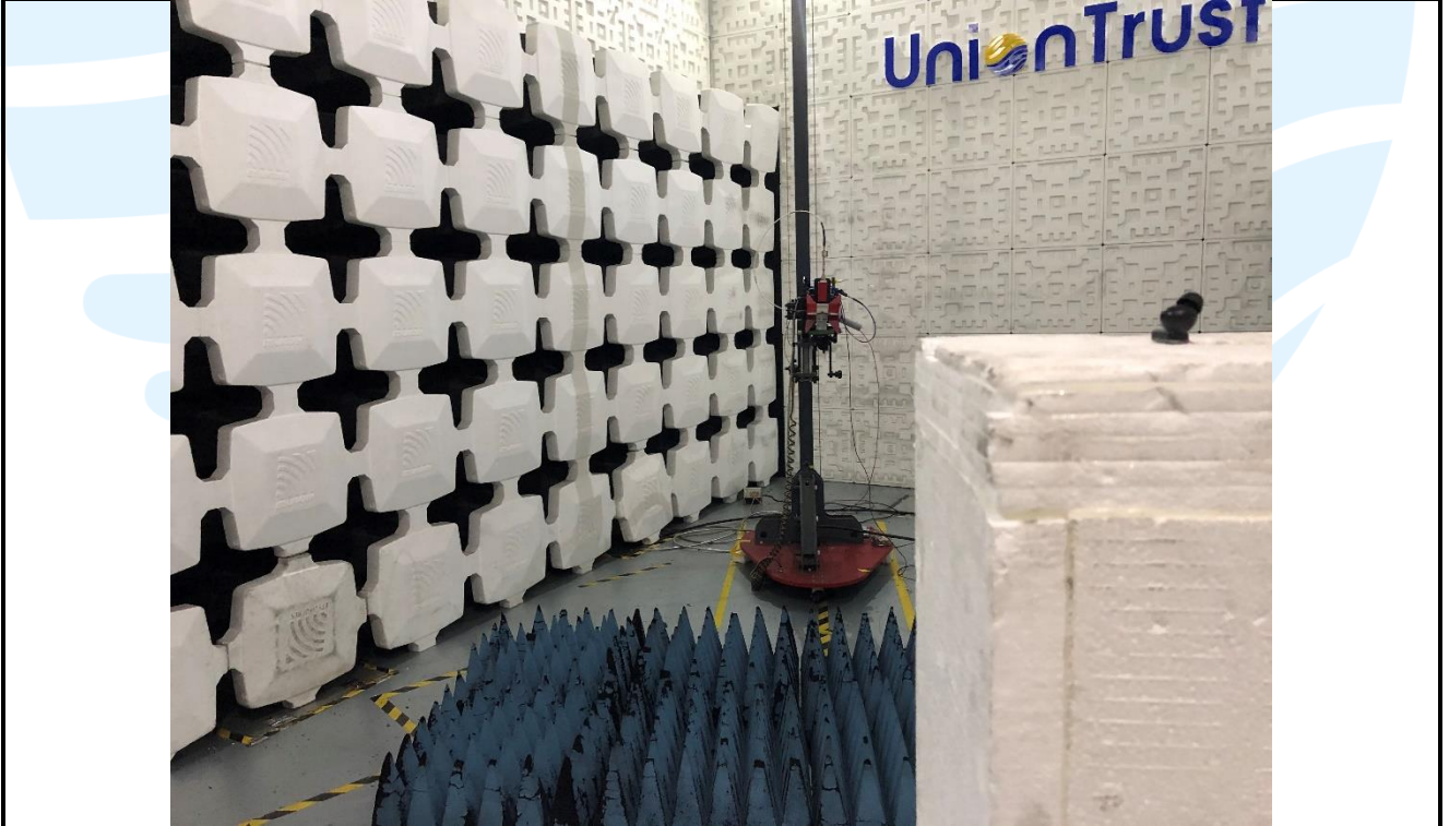
Radiated emission Test Setup (Above 1 GHz) -Right
