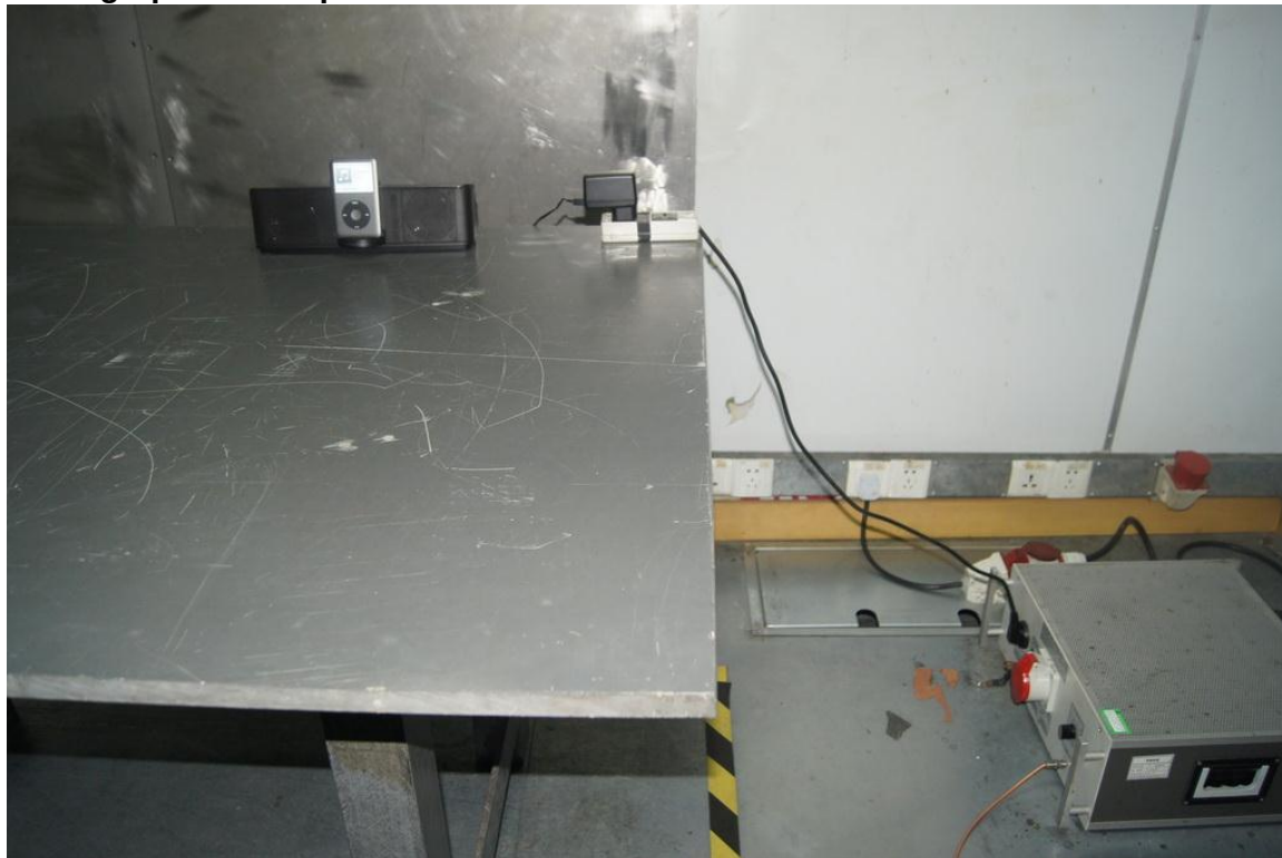
Photograph 2: Set-up for Radiated Emissions
