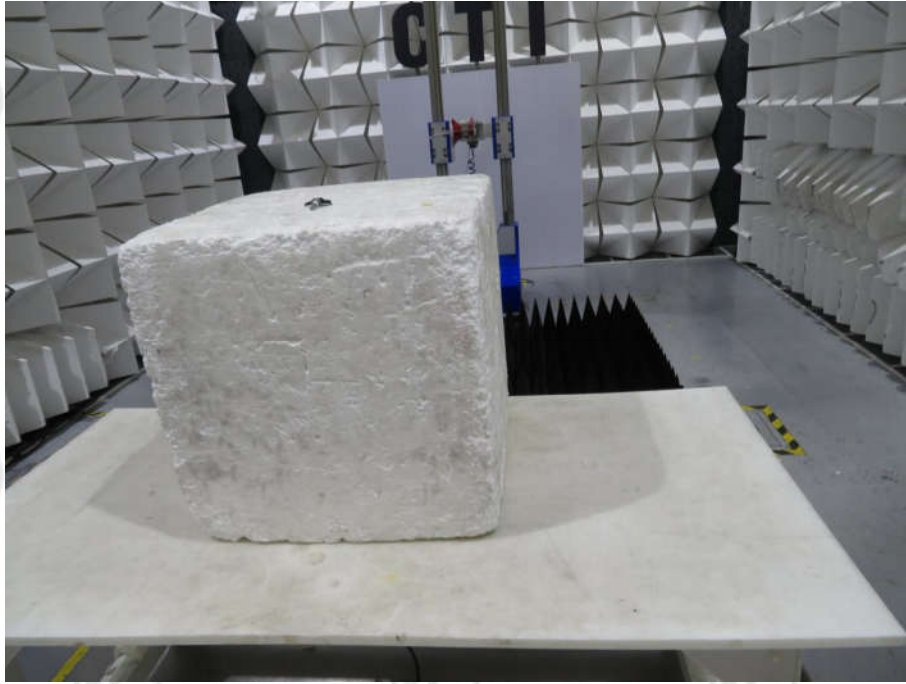
Radiated spurious emission Test Setup-3(Above 1GHz)
