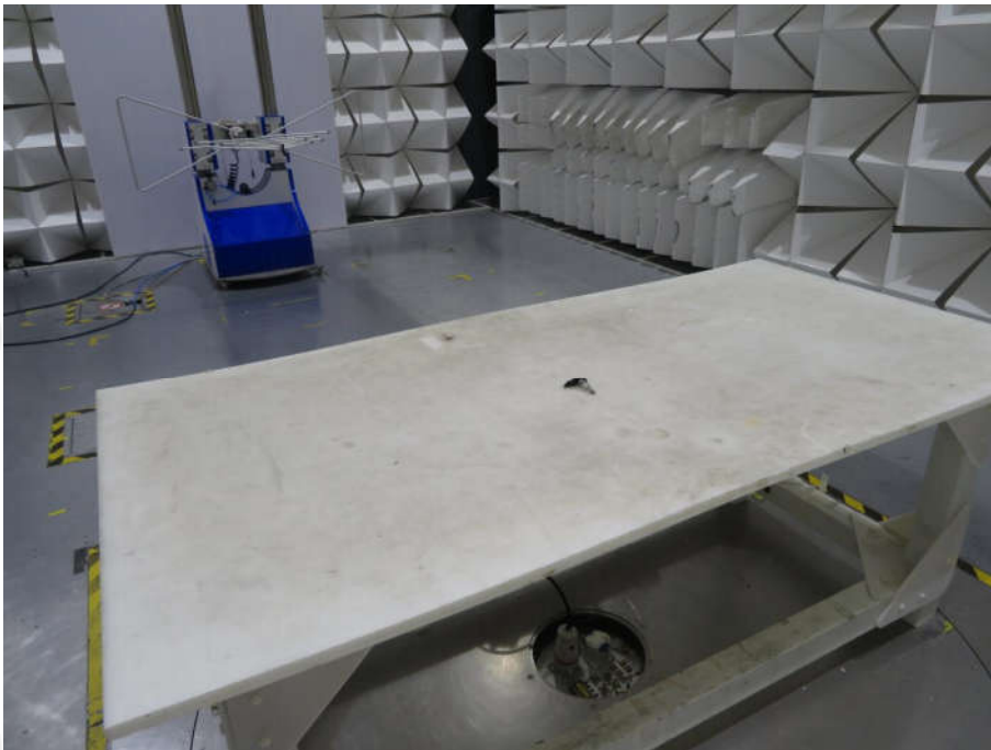
Radiated spurious emission Test Setup-2(30MHz~1GHz)
