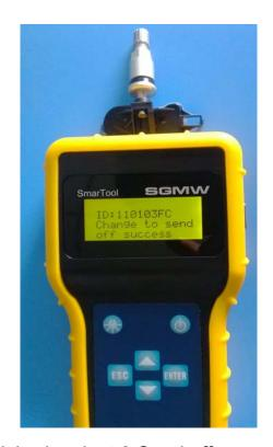
d) when testing finished, select 2.Send off, press ENTER, then shows ID number on the screen of the handle, which means that the transmitter is in dormant state, no data is transmitted then.
