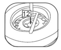
2.4 Final inspection: Visually inspect the rim, valve stem and electronic module to ensure no damage has occurred.
