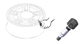
1.3 Take off the nut<sup>®</sup>, insert the valve stem through the rim hole from inside.
