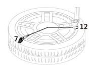
1.6 Mount the upper tire bead the same way. (If the mounting head of the tire changer is positioned at 12 o'clock, then the valve should be at the 5 o'clock position.) Inflate the tire to nominal pressure.
