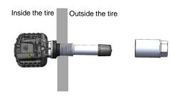
1.4 Place nut<sup>®</sup> on the valve stem, and tighten with  $5\pm$  0.5 N • m (44 inch pounds) torque.
