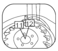
2.3 Use the same procedure to dismount the lower tire bead. (If the mounting head of the tire changer is at the 12 o'clock position, then the valves stem should also be at the 12 o'clock position.)
