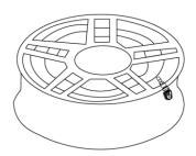
1.5 Lock the rim on the tire changer. (If the mounting head of the tire changer is positioned at 12 o'clock, then the valve should be at the 7 o'clock position.) Apply lubricant on both the tire bead and rim. Mount the lower tire bead on the rim. Ensure that the tire bead does not touch the electronic module during mounting.
