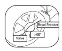
2.2 Firmly fix the wheel on the turntable clamps. (If the mounting head of the tire changer is positioned at 12 o'clock, then the valves stem should be at the 11 o'clock position.) Apply lubricant to both tire bead and rim, and then remove the upper tire bead.
