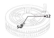
1.7 Apply soapsuds on the valve tip. If no leakage is found, put on the valve cape. If unsuccessful, try again.
