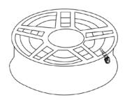
1.5 Lock the rim on the tyre changer. (If the mounting head of the tyre changer is positioned at 12 o'clock, then the valve should be at the 7 o'clock position.) Apply lubricant on both the tyre bead and rim. Mount the lower tyre bead on the rim. Ensure that the tyre bead does not touch the electronic module during mounting.
