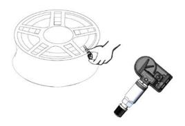
1.3 Take off the nut<sup>®</sup>, insert the valve stem through the rim hole from inside.
