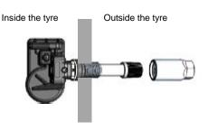
1.4 Place nut<sup>®</sup> on the valve stem, and tighten with 5 Nm (44 inch pounds) torque.
