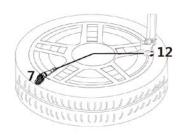
1.6 Mount the upper tyre bead the same way. (If the mounting head of the tyre changer is positioned at 12 o'clock, then the valve should be at the 5 o'clock position.) Inflate the tyre to nominal pressure.
