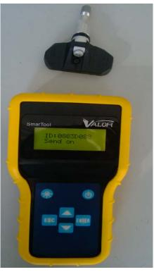
c). After the testing, wake up the tool again to chose "1.Send off" and then press "ENTER" key. When the tool's display shows ID Number and "Send off", it means the sensor is under stationary mode. At this time, it will not send any data (Note: Every time after the test, the sensor should be switched to "Send off").
