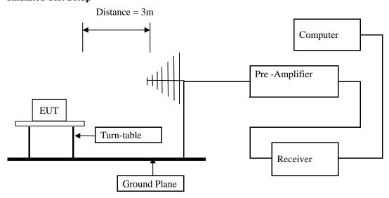
For the actual test configuration, please refer to the related items – Photos of Testing The deactivation test was performed in the 3 meters chamber B test site, using the setup accordance with the ANSI C63.4 - 2003. The specification used was the FCC 15.231(e) limits.
