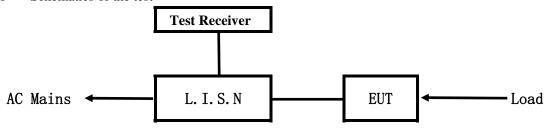
**EUT: Equipment Under Test**
