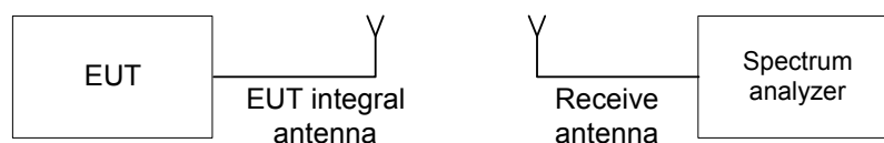
Figure 7.1.1 Setup for transmitter shut down test
