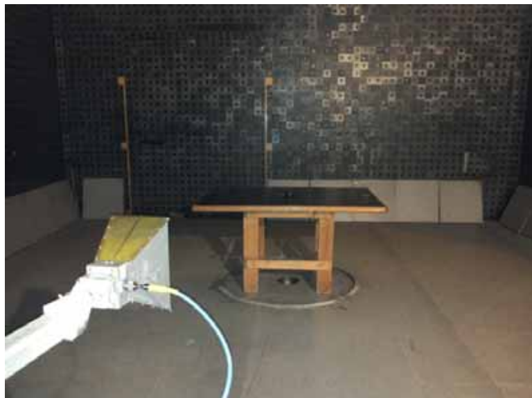
Photograph 8.1.2 Setup for radiated emission measurements
