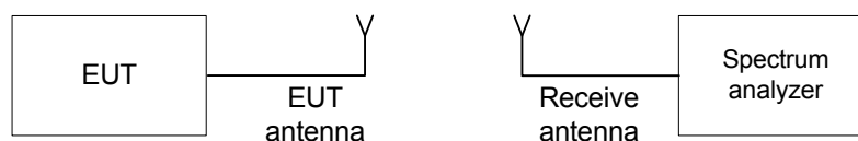
Figure 7.3.1 Occupied bandwidth test setup
