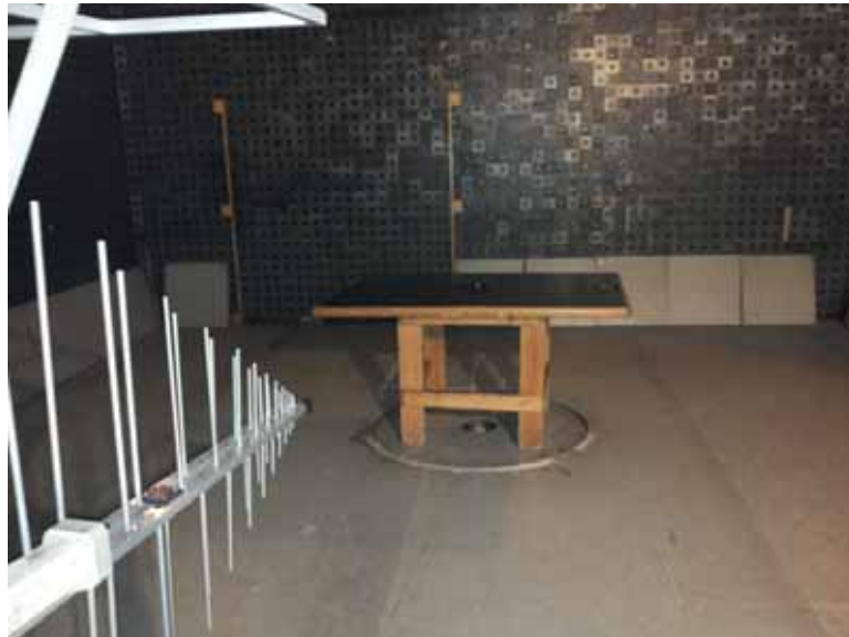
Photograph 8.1.2 Setup for radiated emission measurements
