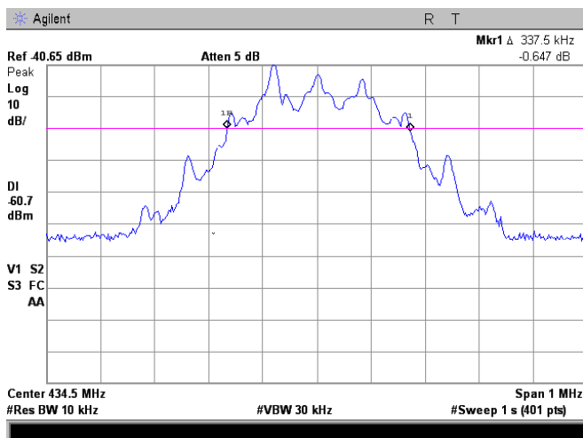
Plot 7.4.4 Occupied bandwidth test result at 434.52 MHz, UHF3 transmitter
