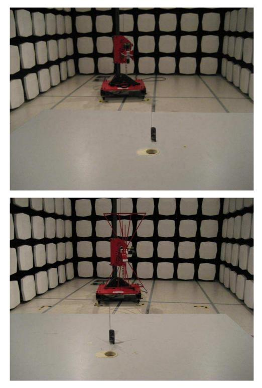
Measurement of Radiated Emission Test Set Up
