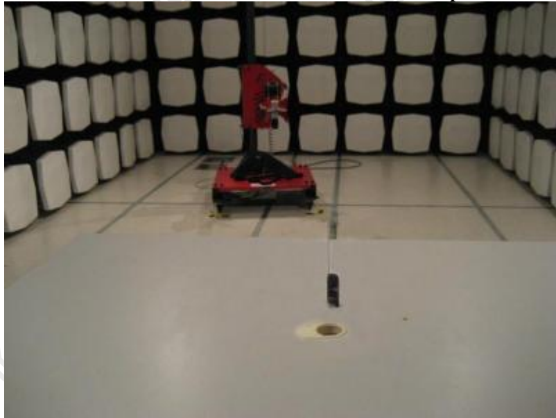
Measurement of Radiated Emission Test Set Up
