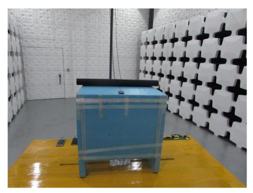
Front View of Radiated Emissions above 1GHz
