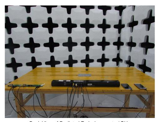
Back View of Radiated Emissions up to 1GHz
