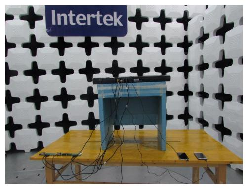
Back View of Radiated Emissions above 1GHz
