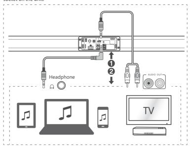
B. Use a 3.5mm to 3.5mm audio cable (included) to connect the TV's or external audio device headphone socket to the **AUX 1** socket on the unit.
