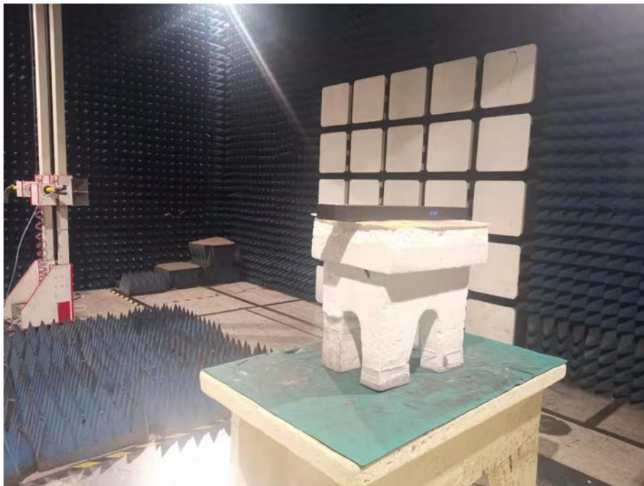
Spurious Emission Test Setup (Above 1GHz)
