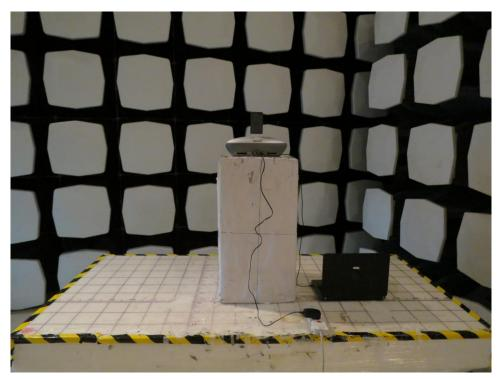
Back View of Radiated Emissions above 1GHz
