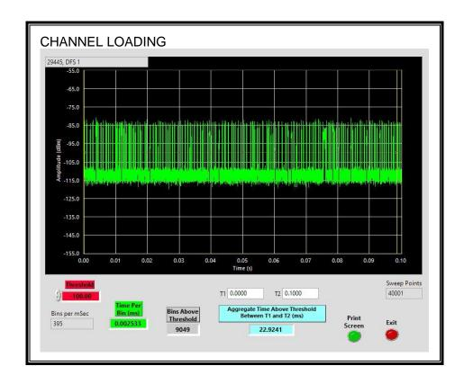
The level of traffic loading on the channel by the EUT is 22.92%
