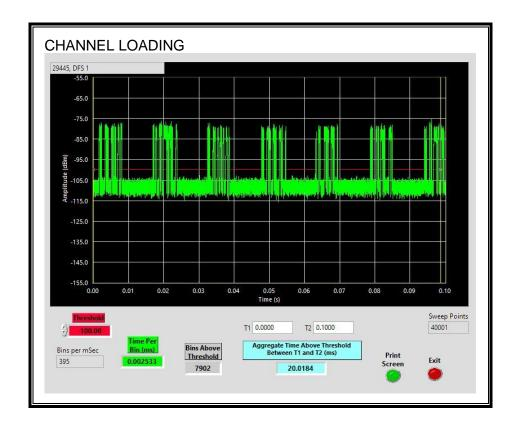
The level of traffic loading on the channel by the EUT is 20.018%
