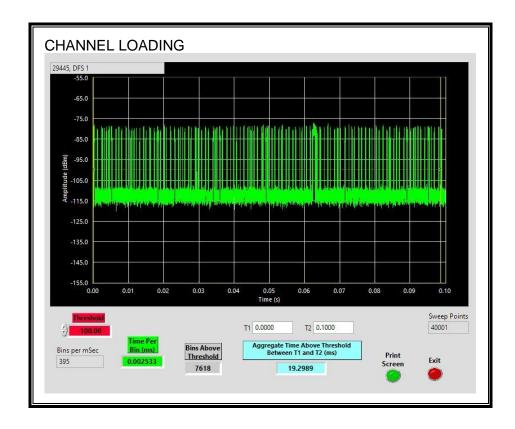
The level of traffic loading on the channel by the EUT is 19.299%
