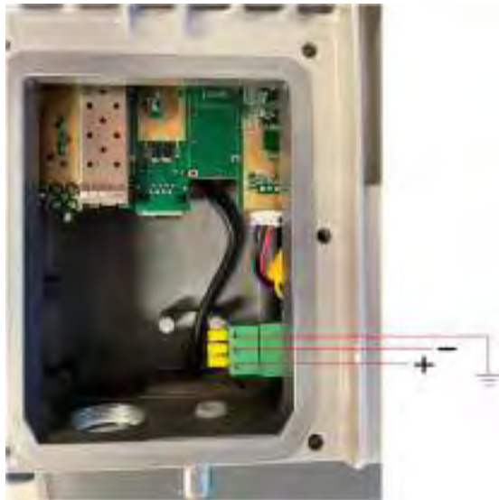
Figure 10 : 3 GHz cnRanger 210 RRH DC power cable
