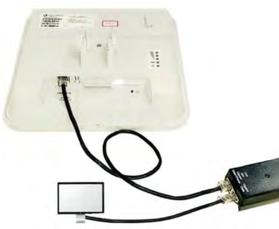
Figure 28 : Installation of Tyndall 101 to PoE adapter
