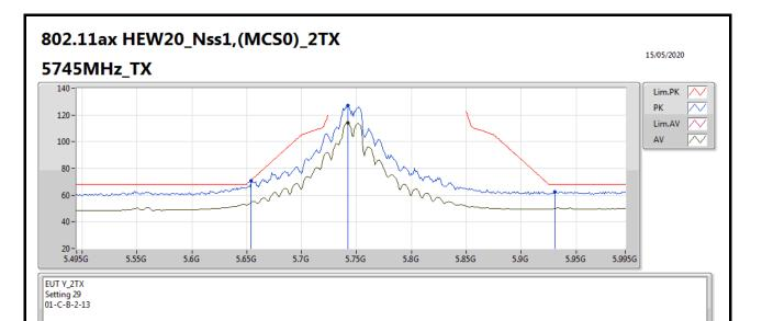
Туре Freq Level Limit Margin Raw Dist Condition Azimuth Height Comment AF CL PA (Hz) (dBuV/m) (dBuV/m) (dB) (dBuV) (dB) (dB) (dB) (m) (m) (°) РК 5.654G 70.60 34.00 6.33 34.70 71.16 -0.56 64.97 Vertical 1.80 19 3 PK 5.742G 126.88 34.13 Inf -Inf 121.05 3 1.80 6.37 34.67 Vertical 19 AV 5.742G 114.34 Inf -Inf 108.51 1.80 34.13 6.37 34.67 3 Vertical 19 5.931G 34.95 34.60 68.20 -5.59 55.79 3 62.61 Vertical 19 1.80 6.47
