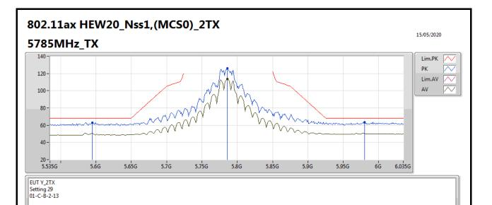
Туре Freq Level Limit Margin Raw Dist Condition Azimuth Height Comment AF CL PA (Hz) (dBuV/m) (dBuV/m) (dB) (dBuV) (dB) (dB) (dB) (m) (m) (°) РК 5.595G 63.09 68.20 57.52 33.99 34.72 Vertical 1.83 6.30 -5.11 22 3 PK 5.786G 126.25 34.26 -Inf 120.25 3 22 1.83 6.39 34.65 Inf Vertical AV 5.786G 113.76 -Inf 107.76 22 1.83 34.26 6.39 34.65 Inf 3 Vertical 5.98G 68.20 22 35.20 34.58 -4.91 6.49 63.29 56.18 3 Vertical 1.83
