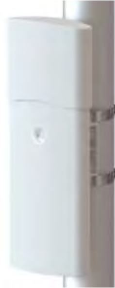
Figure 5 ePMP 3000 Access Point module mounting bracket
