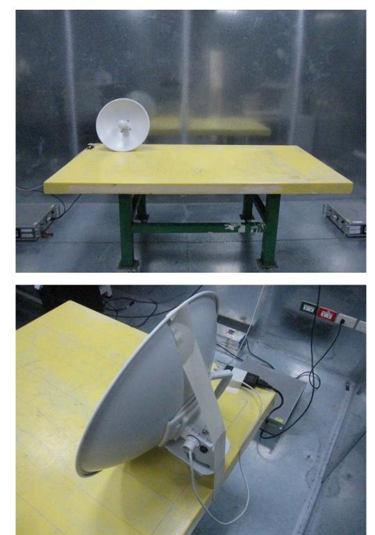
1. Photographs of Conducted Emissions Test Configuration
