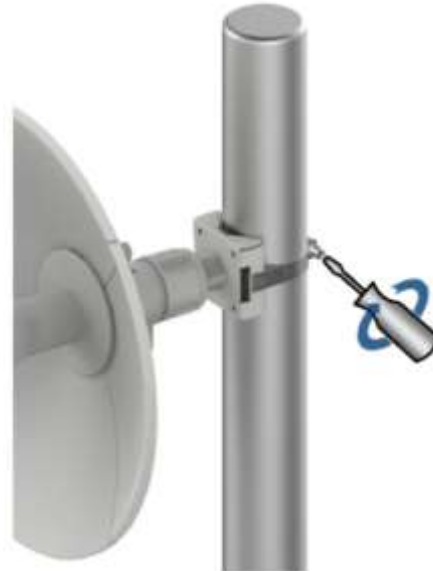
Figure 24 Force 190 mounting bracket (clamp securing)
