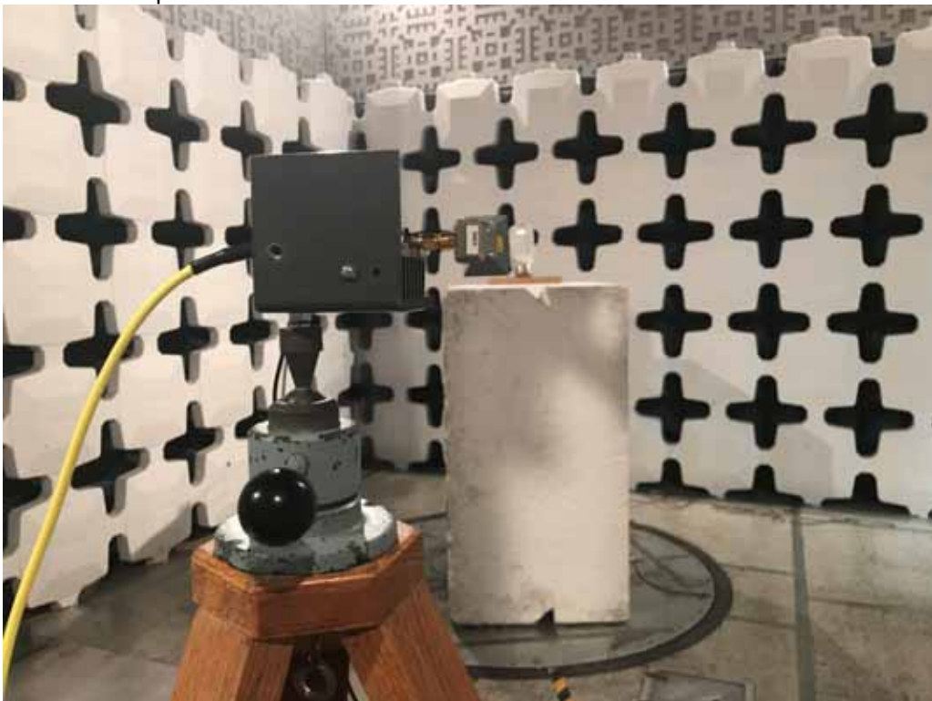
Test Setup for Radiated Emissions above 18-26GHz – Vertical Polarization
