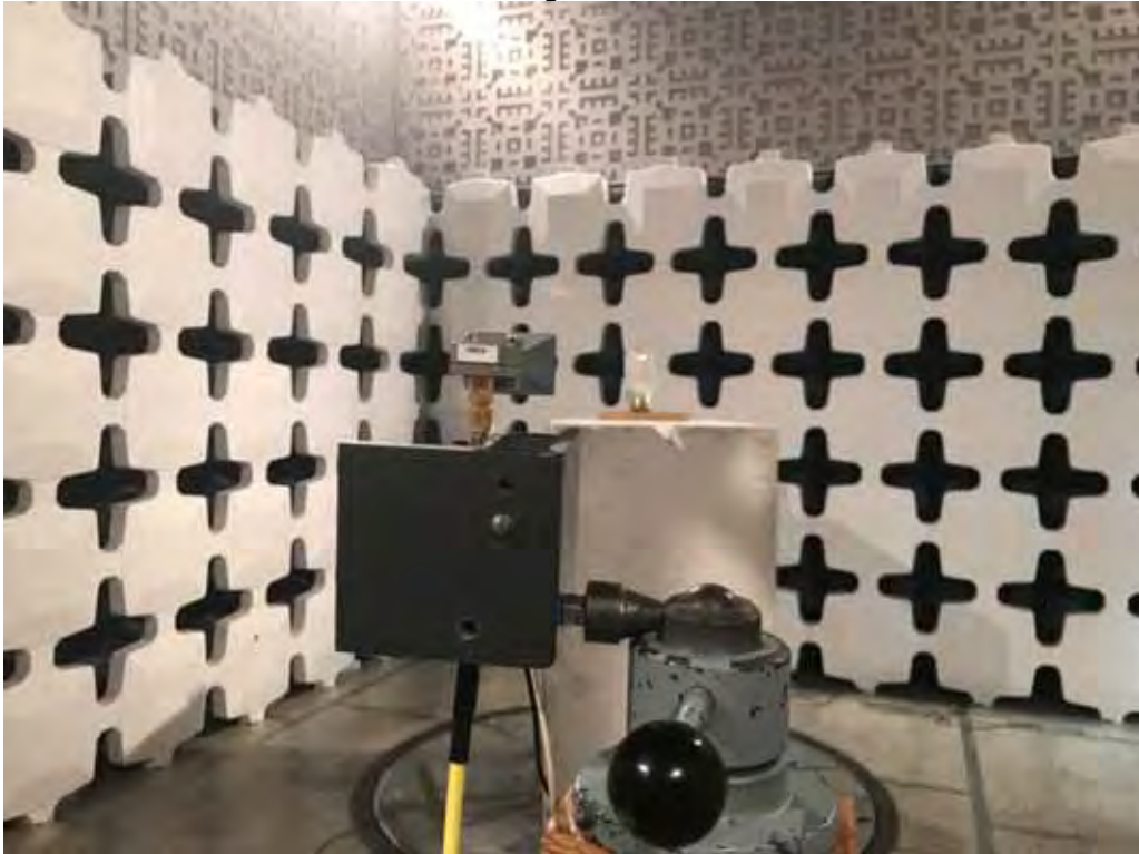
Test Setup for Radiated Emissions above 18-26GHz – Horizontal Polarization
