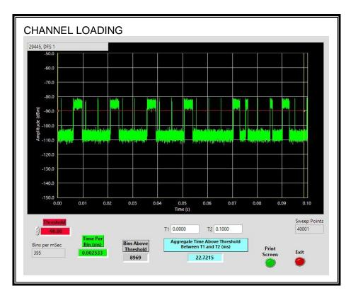
The level of traffic loading on the channel by the EUT is 22.72%
