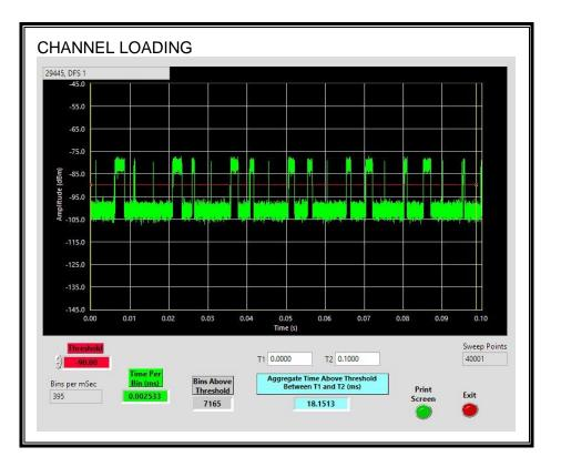
The level of traffic loading on the channel by the EUT is 18.15%
