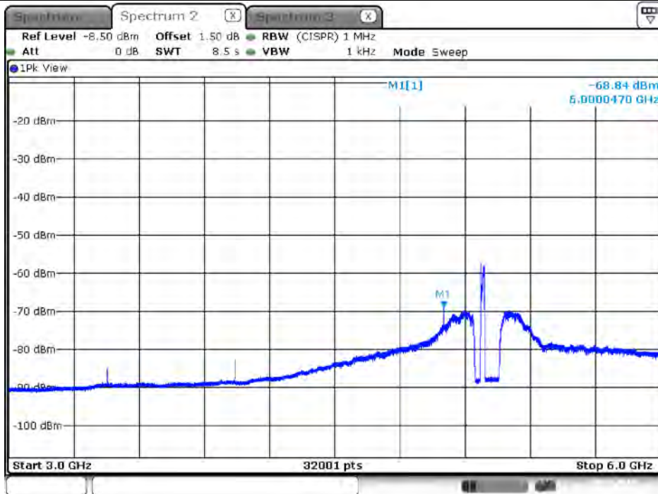
Plot on Configuration VHT20 / 5180 MHz / Average / Port 3 / 3GHz~6GHz
