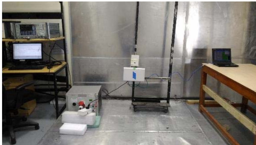
Figure 15 Test setup for Conducted Emission test 150 kHz to 30MHz
