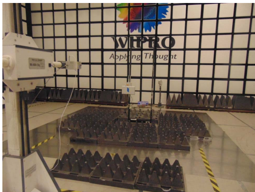
Figure 14 Test setup for Radiated Emission test from 26.5GHz to 40GHz – Vertical Polarization
