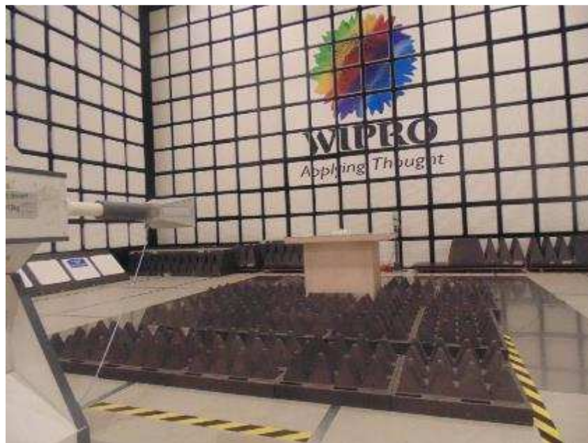
Figure 10: Test setup for Radiated Emission Test from 1 GHz to 18 GHz – Vertical Polarization
