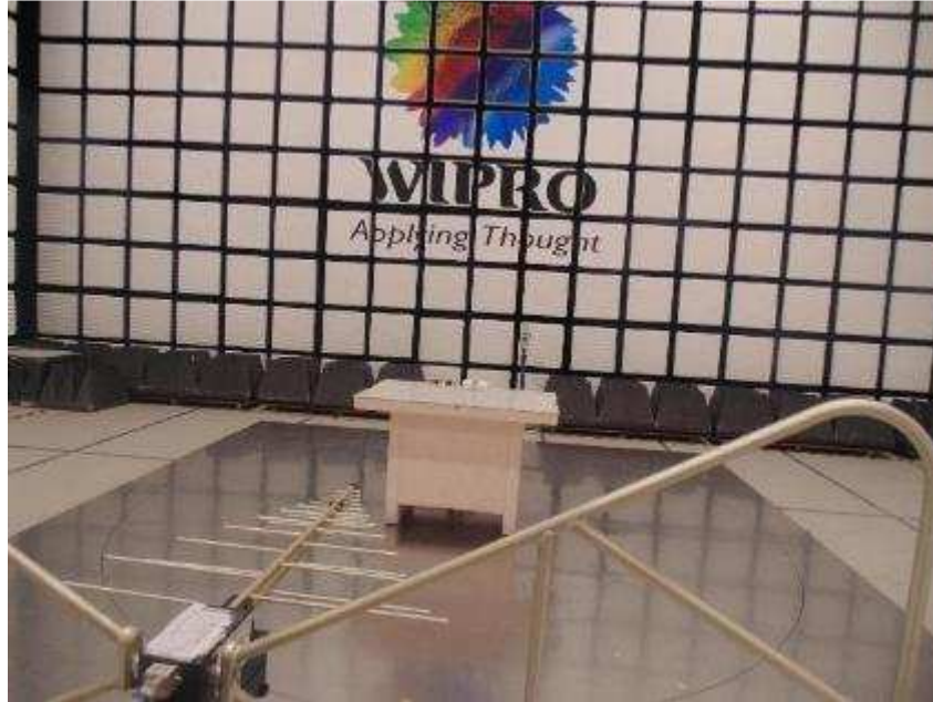
Figure 7: Test setup for Radiated Emission test from 30MHz to 1GHz - Horizontal Polarization
