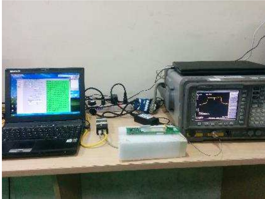
Figure 15: Conducted RF Test set up photograph
