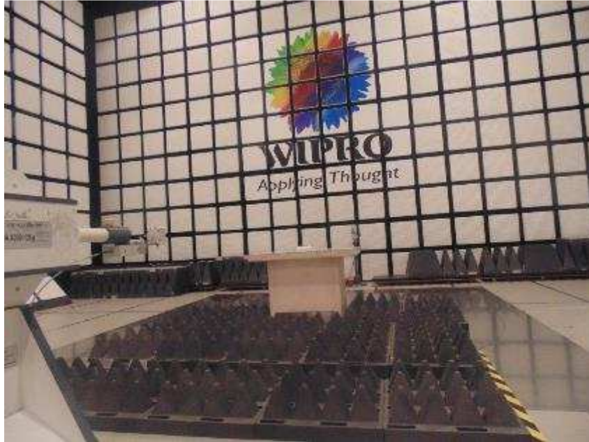
Figure 11: Test setup for Radiated Emission Test from 18 GHz to 26.5 GHz – Horizontal Polarization
