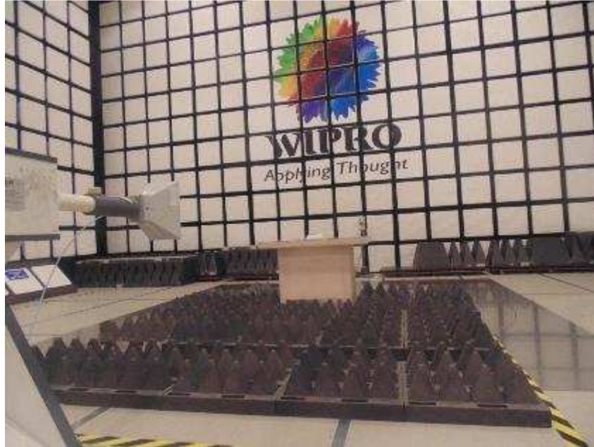
Figure 9: Test setup for Radiated Emission Test from 1 GHz to 18 GHz – Horizontal Polarization
