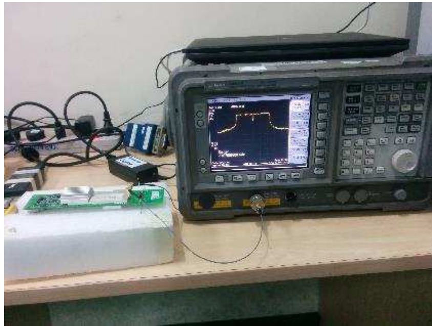
Figure 16 Conducted RF Test set up photograph
