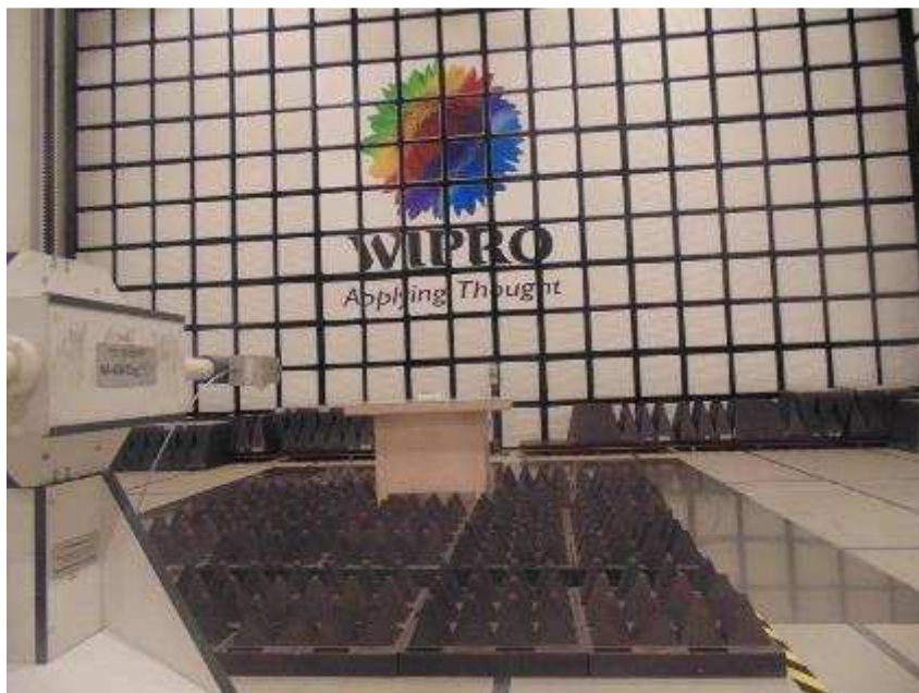
Figure 12: Test setup for Radiated Emission Test from 18 GHz to 26.5 GHz – Vertical Polarization
