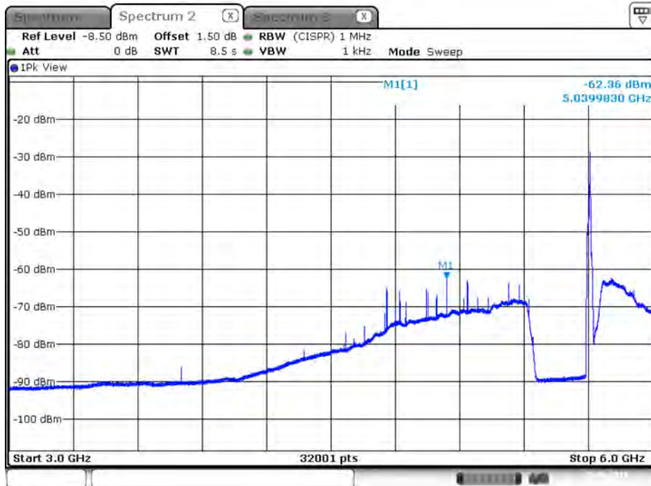
Plot on IEEE 802.11ac Nss1 MCS0 VHT20 / 5700 MHz / Average / Port 1 / 3GHz~6GHz
