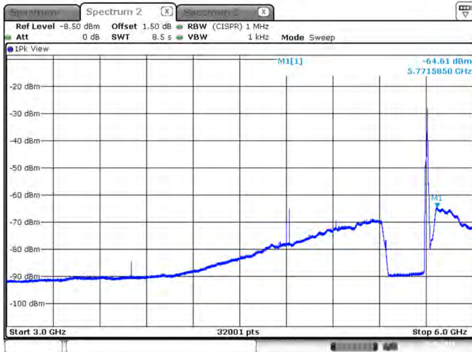
Plot on IEEE 802.11ac Nss1 MCS0 VHT20 / 5700 MHz / Average / Port 2 / 3GHz~6GHz
