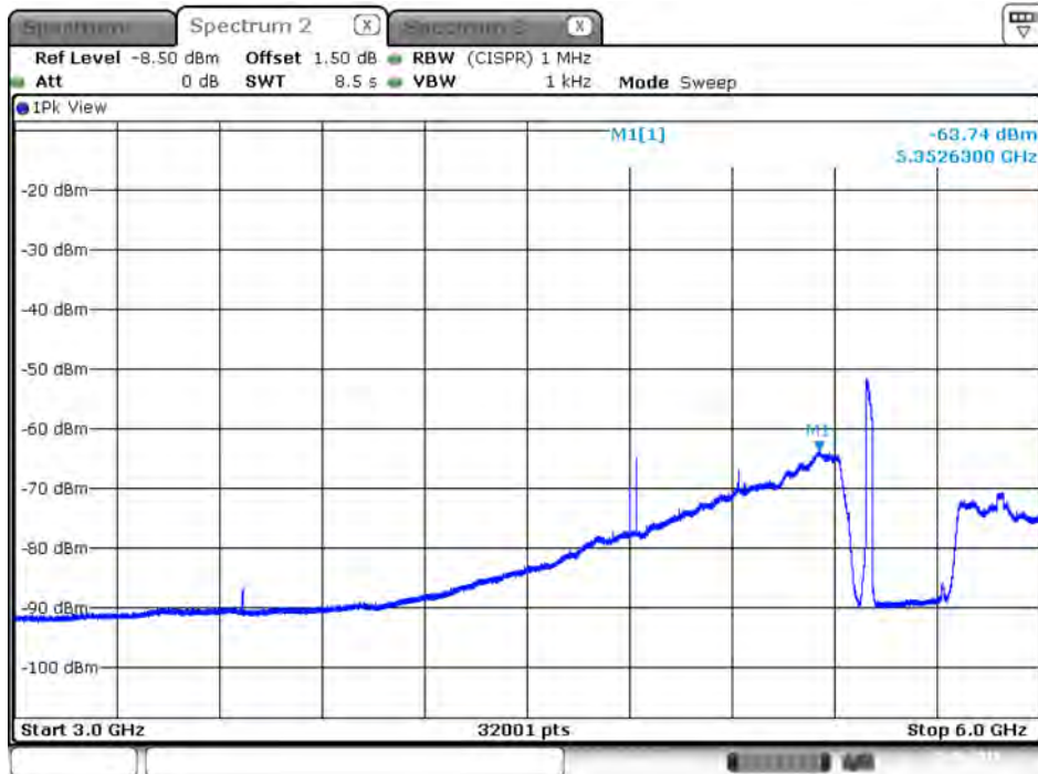
Plot on IEEE 802.11ac Nss1 MCS0 VHT20 / 5500 MHz / Average / Port 2 / 3GHz~6GHz
