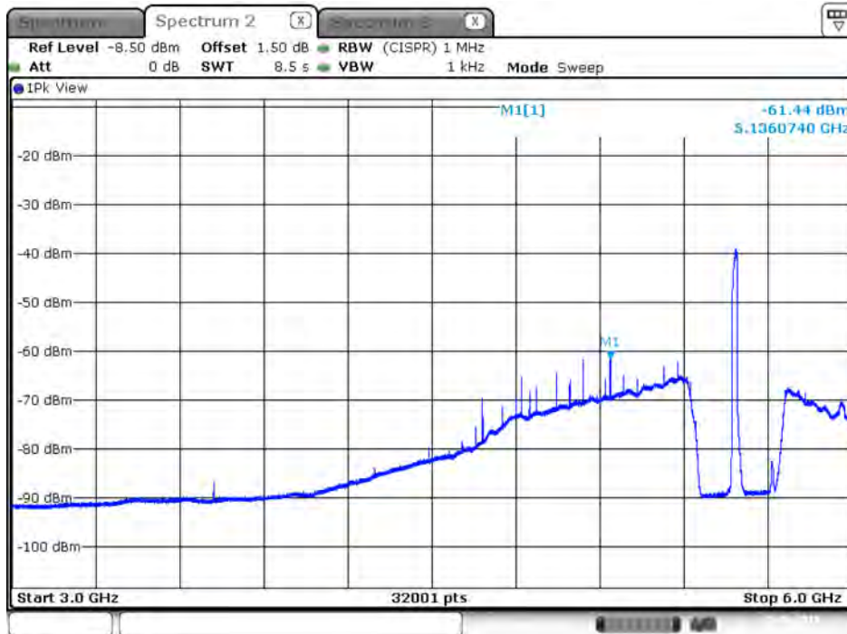
Plot on IEEE 802.11ac Nss1 MCS0 VHT20 / 5580 MHz / Average / Port 1 / 3GHz~6GHz
