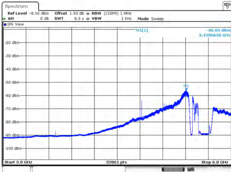
Plot on IEEE 802.11ac Nss1 MCS0 VHT80 / 5530 MHz / Average / Port 2 / 3GHz~6GHz
