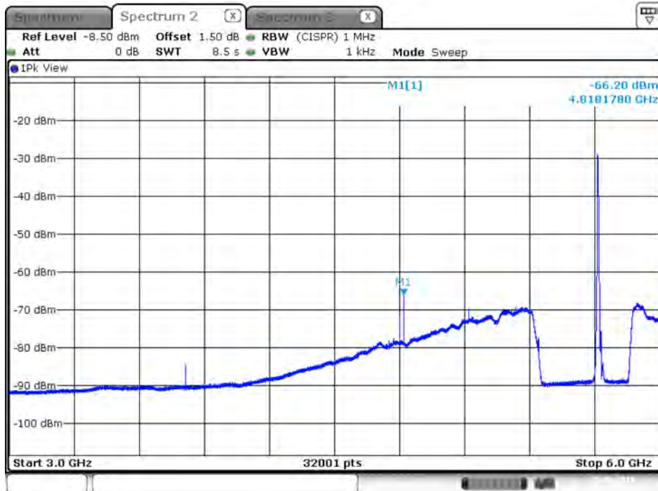
Plot on IEEE 802.11ac Nss1 MCS0 VHT20 / 5720 MHz / Average / Port 2 / 3GHz~6GHz
