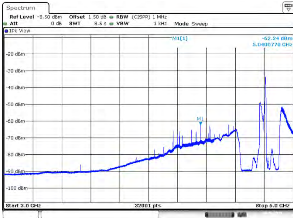
Plot on IEEE 802.11ac Nss1 MCS0 VHT80 / 5690 MHz / Average / Port 2 / 3GHz~6GHz
