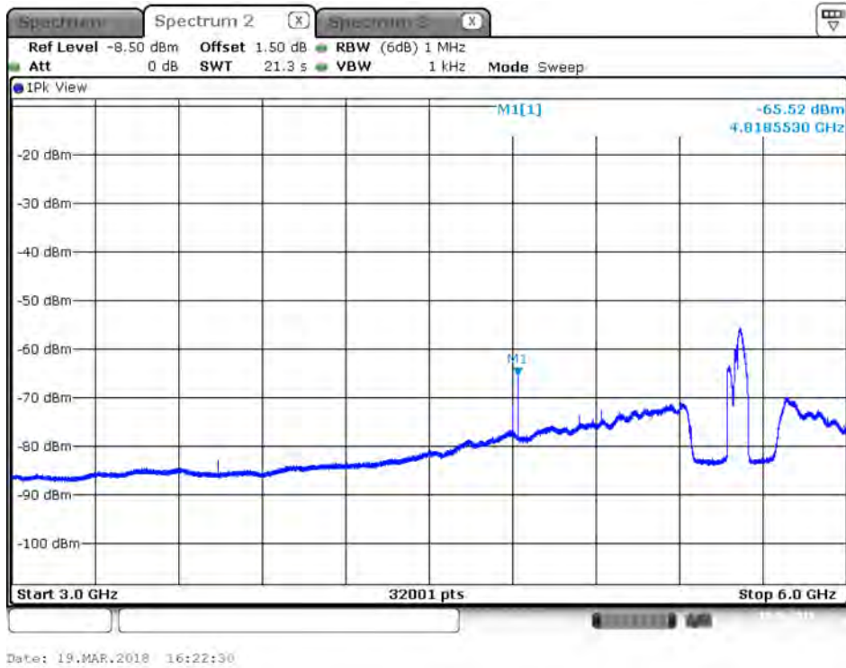
Plot on IEEE 802.11ac Nss1 MCS0 VHT80 / 5610 MHz / Peak / Port 2 / 3GHz~6GHz
