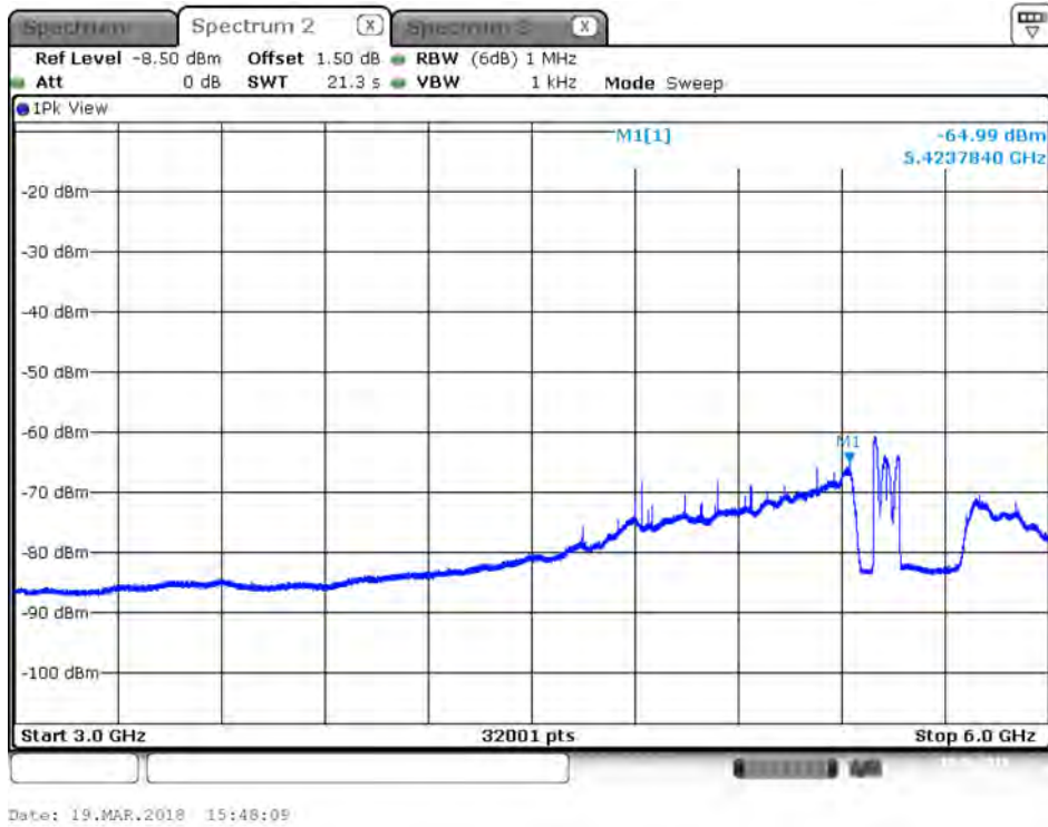
Plot on IEEE 802.11ac Nss1 MCS0 VHT80 / 5530 MHz / Peak / Port 1 / 3GHz~6GHz
