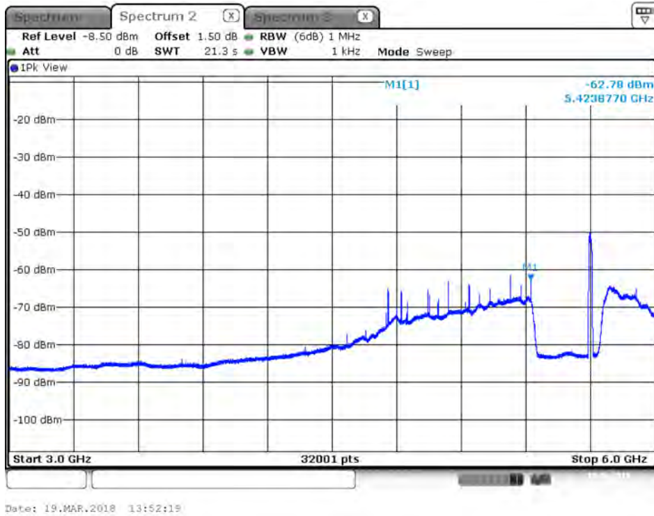
Plot on IEEE 802.11ac Nss1 MCS0 VHT20 / 5700 MHz / Peak / Port 1 / 3GHz~6GHz
