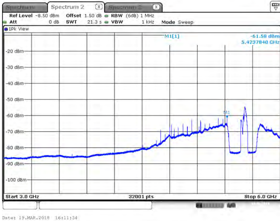
Plot on IEEE 802.11ac Nss1 MCS0 VHT80 / 5610 MHz / Peak / Port 1 / 3GHz~6GHz
